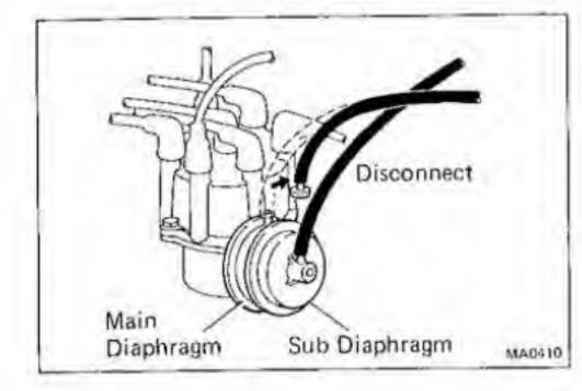
(b) Disconnect the hose from the distributor main diaphragm and plug the hose end. This will cut the vacuum advancer.
